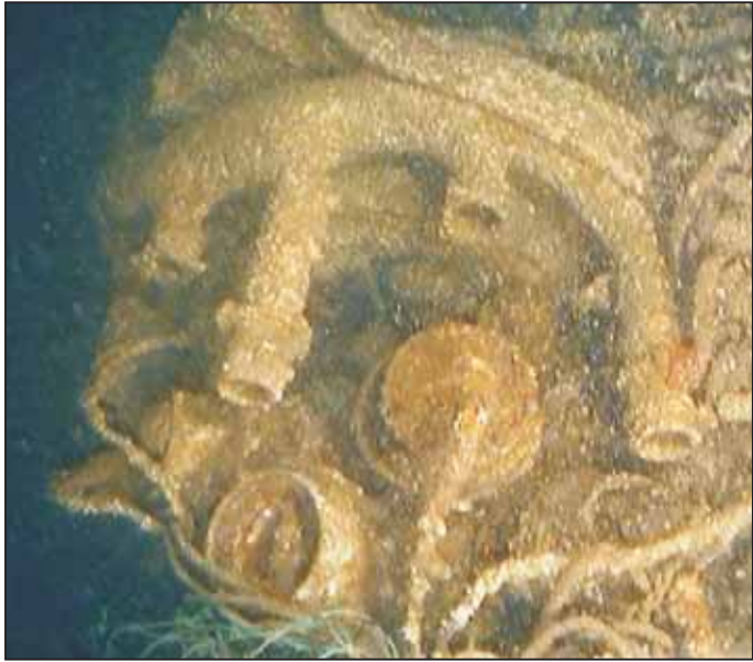
Plate C: Details of cylinders and exhaust collector ring on engine 2.
