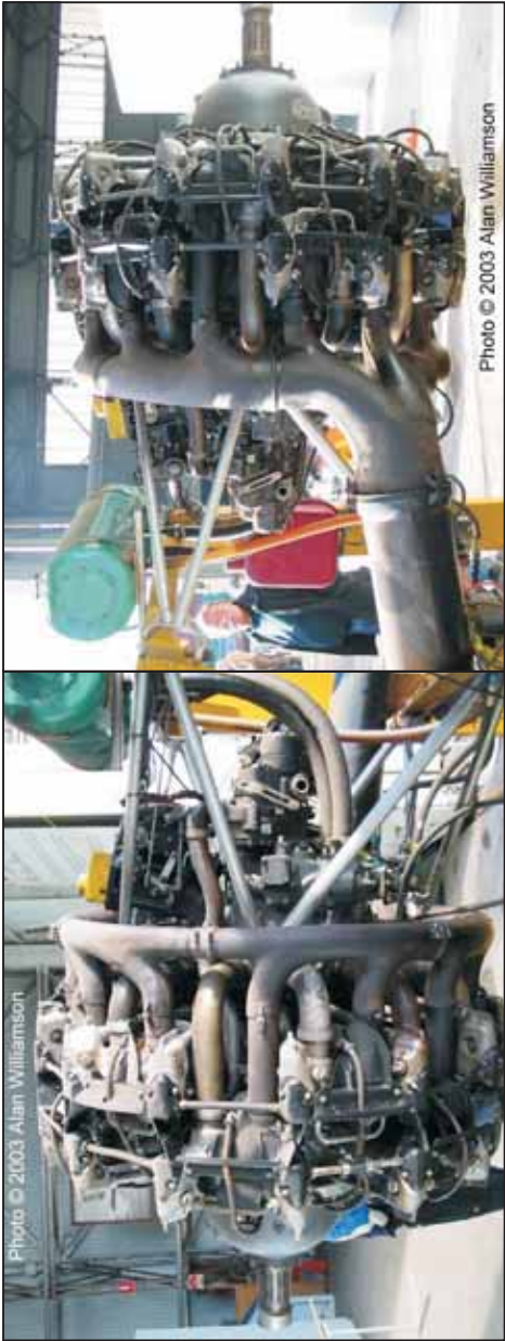
Plate A: Photographs of a Pratt & Whitney R-1830 Twin Wasp engine
